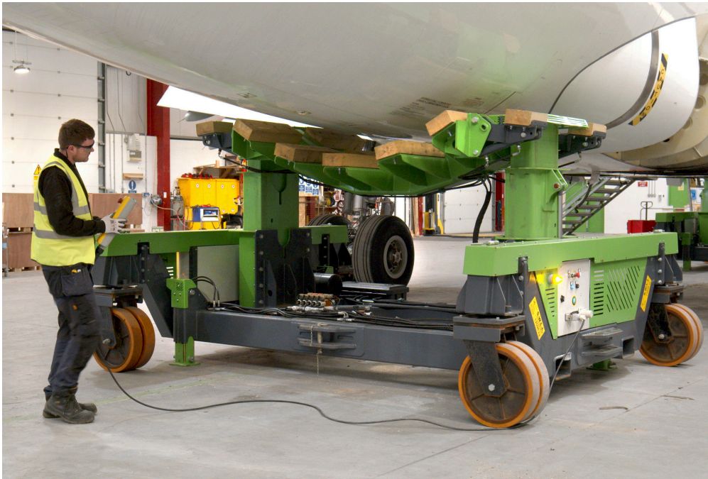
CLOCKWISE FROM TOP LEFT: EirTrade Aviation has become the leading independent supplier of Boeing 787-8 parts to the industry All images via EirTrade A specially designed cradle allows the undercarriage to be removed at the start of the teardown process EirTrade Aviation's headquarters is located in Rathcoole, County Dublin, Ireland Engine stand leasing and sales have become a significant part of EirTrade Aviation's current business
